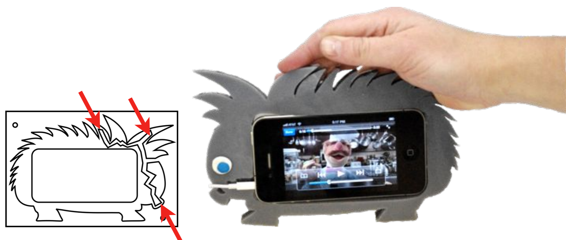
Interactive iPhone case. Stroke the downward-facing fur for “volume down”, and the upward-facing fur for “volume up”. Push its nose for “play/pause”. The mold slice shows the location of the hidden switches.
