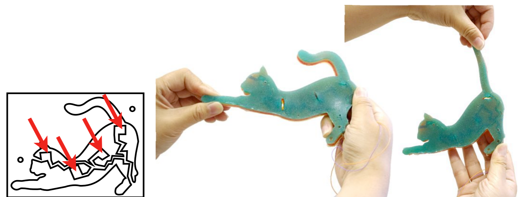
Cat Stretch! A simple cat toy giveaway. Switches embedded in its silicone body register where the cat is stretching, turning a hard continuous problem into a discrete one.
