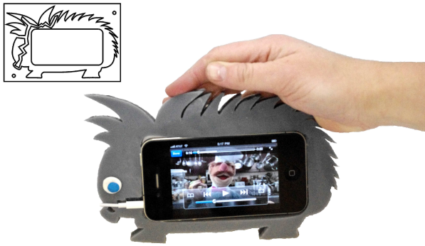
Figure 14. A user turning down the volume with the cellphone guinea pig case. The diagram of a mold slice shows the routing to the three switches.
