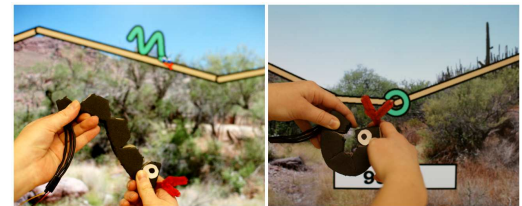
Figure 10. The bend sensor as snake controller.
